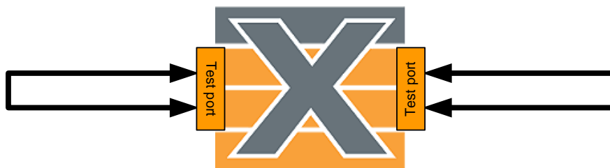
Figure 10. Calibrating test ports in local loop-back mode.
