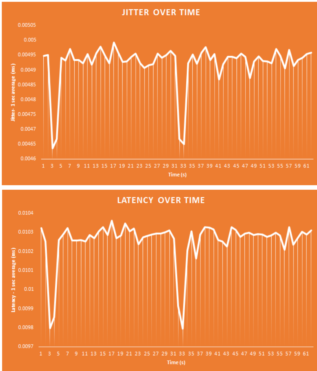
Figure 8. Latency and jitter – 1 sec average over time
